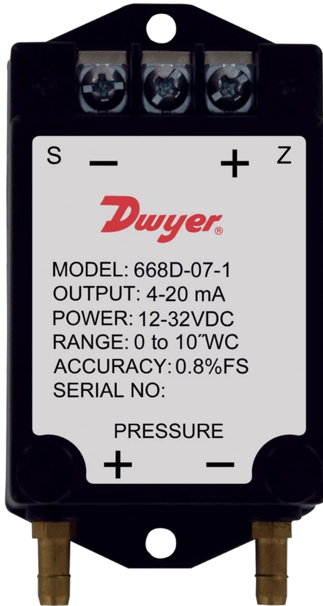
Differential Pressure Transmitter, Compact Ranges from 0.1 to 100 in w.c. Overpressure Protection to 15 psig, \pm 0.8\% Accuracy
